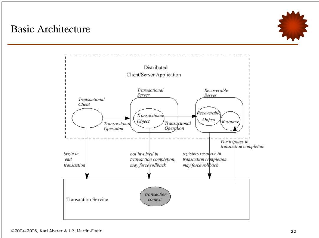
For understanding the transaction service specification one needs first to understand the relevant entities (objects) that participate in a distributed transactional application. To that end one distinguishes three types of objects: transactional clients, transactional servers, and recoverable servers. One can think of these three types of object as corresponding to the three layers of a three-tier architecture.
