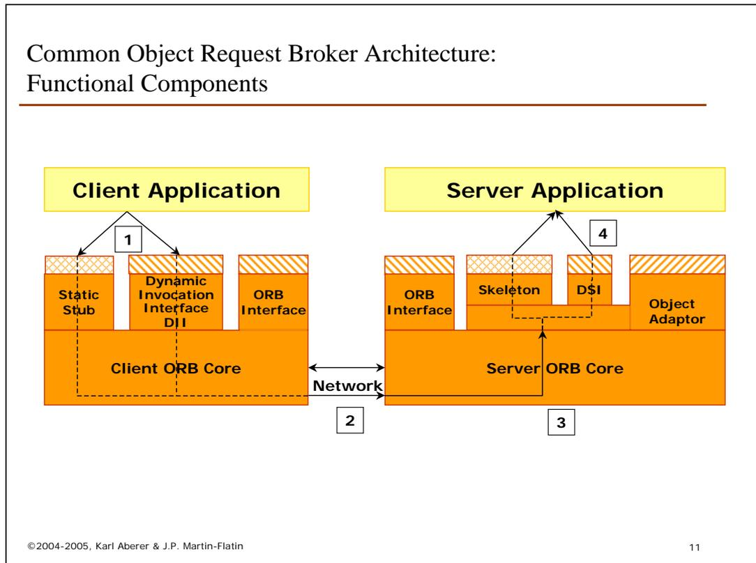
This figure depicts the functional components that an ORB needs in order to forward a request from the client to the server. The client has access to three interfaces of the ORB:
